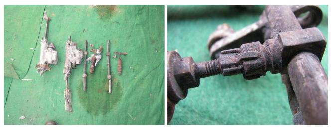
Figure 17: Fire damaged hydraulic servos (L) and wiredrive locking tabs and nuts on a servo (R)
