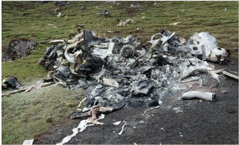
Figure 5: Burnt fuselage
