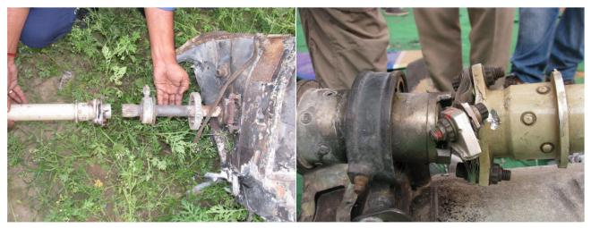
Figure 14: Aft Aluminium driveshaft (L) and Overload Fractured coupling ears (R)
