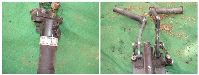
Figure 16: Throttle Position at FLY position (L) and Tail rotor pedals (R)
