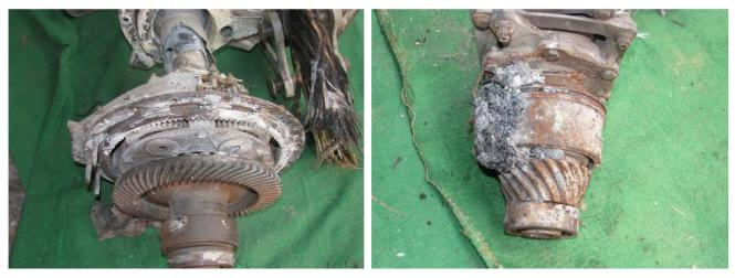
Figure 8: Burnt Main Transmission casing, Intact Planetary Gears and Spiral Bevel Gear (L) Input Quill Gear (R)
