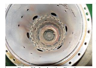
The inner combustion liner was undamaged, exhibited no cracking, thermal damage or evidence of abnormal combustion, such as streaking (Fig 22). Metallic spatter was distributed around the forward end of the combustion liner.
