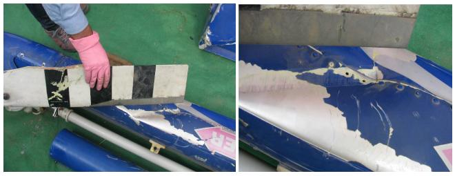
Figure 7: Tail Rotor contact marks on left side of tailboom
