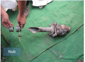
Figure 9: KaFlex main driveshaft and Nub t
