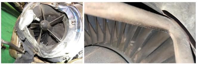
Figure 21: Engine inlet (LH) and 4<sup>th</sup> Stage Power Turbine Blades (RH)
