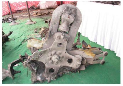
Figure 11: Main Rotor Hub
