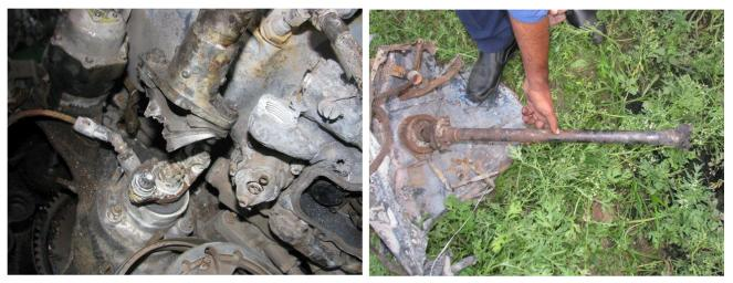
Figure 13: Fractured flexible Thomas Coupling (L) and aft end of fire damaged steel tail rotor drive shaft (R)
